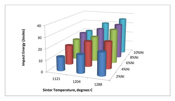
**Figure 5**. Effect of Ni Content and Sintering temperature on Impact Energy. Constant C level of 0.65%.
