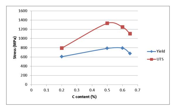
**Figure 10**. Effect of C level on the UTS and yield strength; Ni level fixed at 8%. The 0.65% C test samples were molded at 552 MPa (40 tsi), while all others were molded at 690 MPa (50 tsi).
