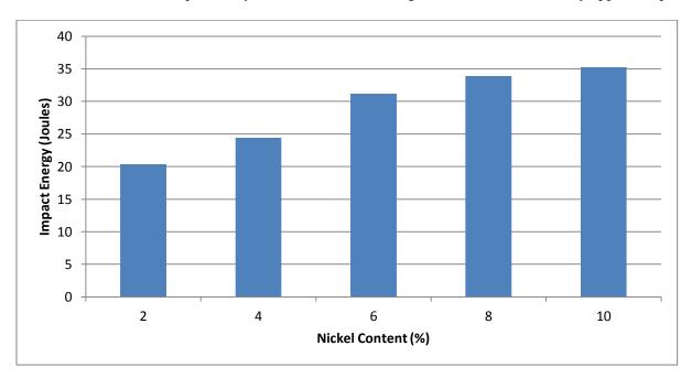
**Figure 7.** Effect of Ni content on Impact Properties; C level fixed at 0.65% and sintering temperature of 1288 °C (2350 °F),
