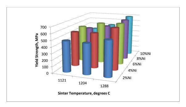
**Figure 4**. Effect of Ni content and sintering temperature on Yield Strength. Constant C level of 0.65%.
