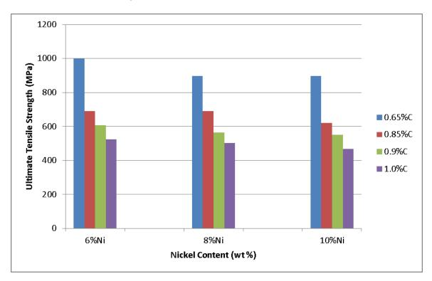
**Figure 8**. Effect of Ni and C level on UTS after sintering at 1274  $^{0}$ C (2325  $^{0}$ F).
