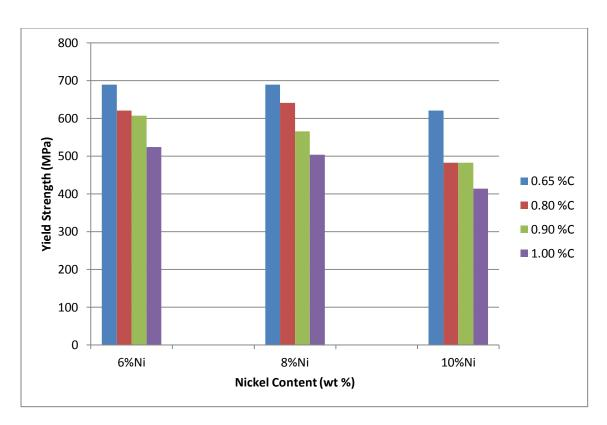
**Figure 9**. Effect of Ni and C level on yield strength after sintering at 1274  $^{0}$ C (2325  $^{0}$ F).
