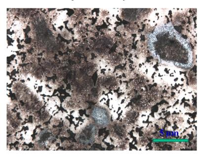
**Figure 12**, Typical microstructure of the Fe-8%Ni-0.5%C-0.85%Mo alloy; consisting of martensite, lightly-etched nickel-rich areas, upper/lower bainite and pearlite. Original magnification 200x. 2 % nital etch.
