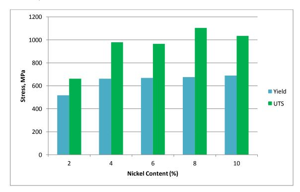
**Figure 6**. Effect of Ni content on UTS and Yield Strength; C level fixed at 0.65% and a sintering temperature of 1288  $^{0}$ C, (2350  $^{0}$ F).
