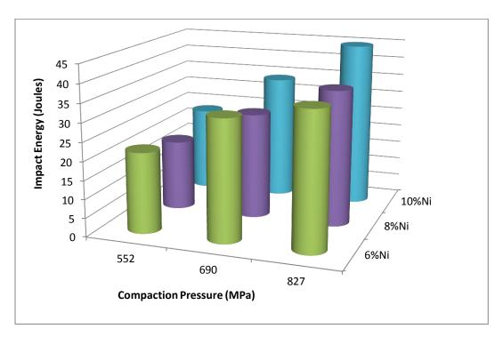
**Figure 11**. Effect of Compaction Pressure and Ni content on Impact Energy. Constant sintering temperature (1288  $^{0}$ C, 2350  $^{0}$ F) and C content (0.5 %).
