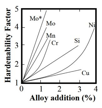
**Figure 1.** Hardenability factors for selected pre-alloyed elements in Fe.<sup>1</sup> Mo\* is the hardenability factor of the element for Ni contents>0.75 wt.%.
