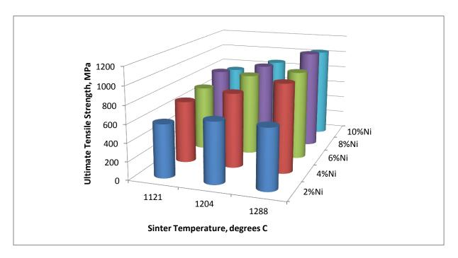
**Figure 3**. Effect of Ni content and sintering temperature on Ultimate Tensile Strength (UTS). Constant C level of 0.65%.
