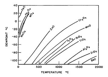
**Figure 2.** The equilibrium temperature for reduction of selected metal oxides as a function of hydrogen dew point; components in assumed to be in pure, standard, states.<sup>6</sup>
